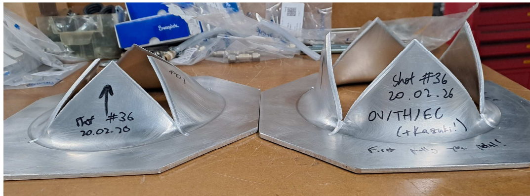
Aluminium 1050-H14. 5.0mm thickness, 2.0mm score depth First fully open petals on downstream diaphragm (right)
