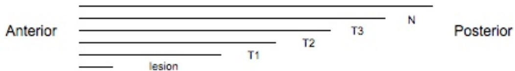
Figure 3-6 - Template 1. This template was used to sample the cross sections of AKA specimens. The lesion refers to the equivalent region to full thickness cartilage loss in AMG. T1 – T3 are equal thirds of the equivalent of damaged cartilage in AMG, and N is the equivalent of the undamaged cartilage in AMG.
