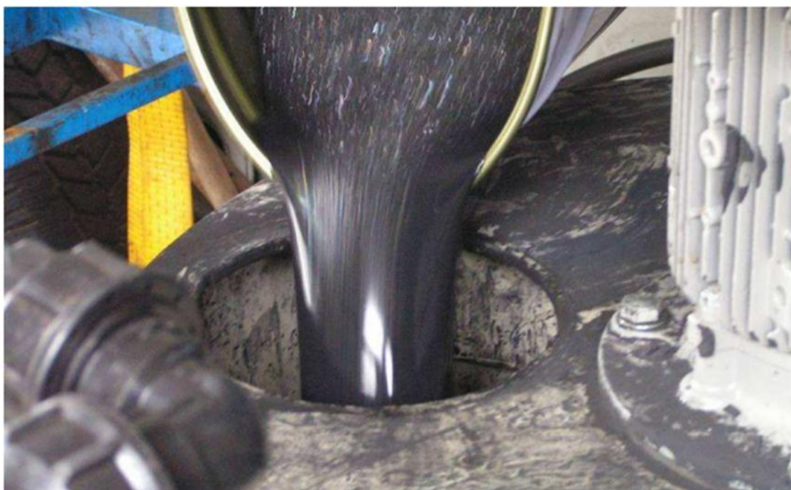
Figure 4.17: Ex-situ slurry reactor with nano-scale iron particles employed in remediation of wastewater. (Observatory NANO focus report 2010).
