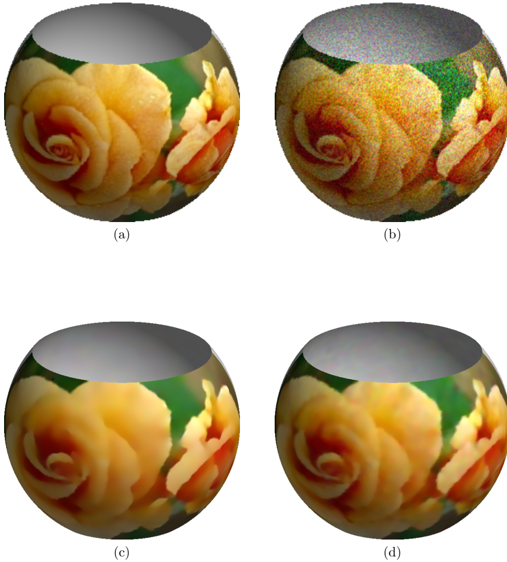
Figure 6.6: Perona–Malik and total variation diffusion on a colour image. Original surface image (a), image with noise in the embedding space (b), result of Perona–Malik denoising (c), and result of total variation denoising (d). Parameters used are \Delta x = 0.007 , \lambda_{PM} = 2 , \lambda_{TV} = 10 . Photo courtesy of Toni Lanker.
