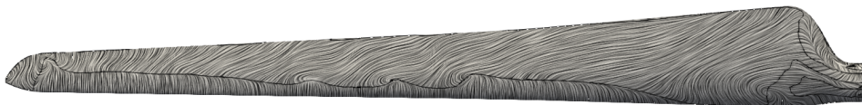
Figure 5.4: Streamlines over the suction surface of the MEXICO rotor plotted using the line integral convolution technique, with the black line highlighting the approximate location where separation occurs. The three analysed tip-speed ratios are displayed.
