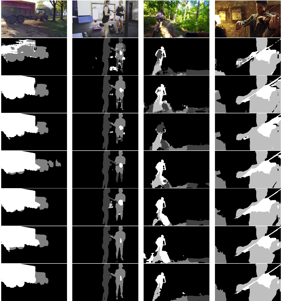
Figure 6.4.4: The impact of successive interactions on the quality of the segmentation outputs. The top row illustrates the input images and the segmentation results for consecutive interactions are depicted in the 2nd to 8th rows.
