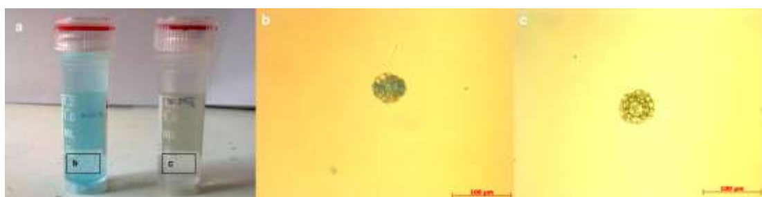
Figure 4.11 Images of porous MS after Alcian Blue staining (a) optical images of (b) heparin coated and (c) control MS (NaOH modified without immersion in heparin). Heparin, stained blue, was only found on (b) the heparin coated MS.
