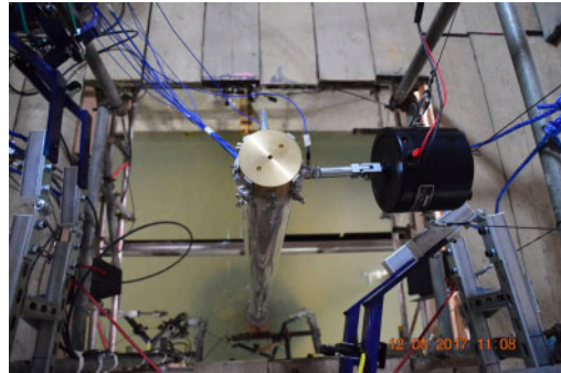
Figure 10. Modal shaker attached to the top of the tower.
