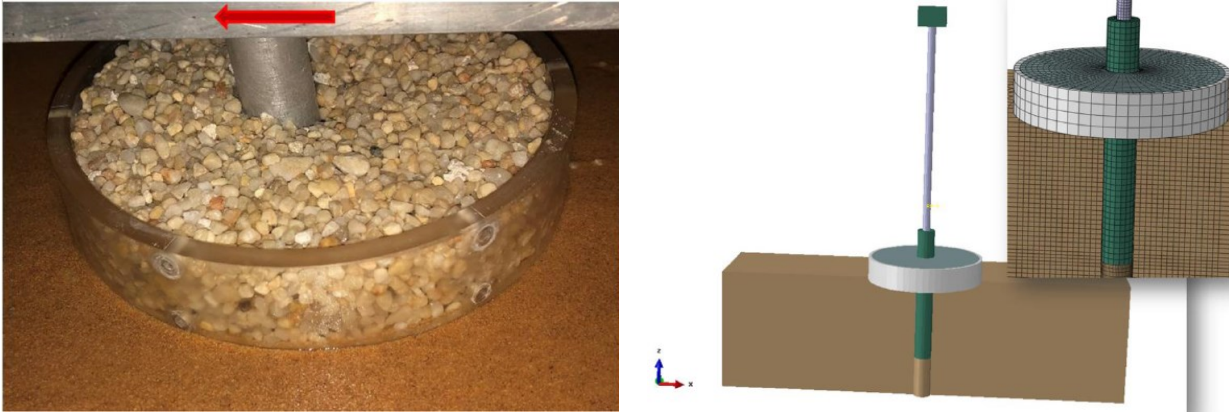
(a) (b) Figure 1.29. Modelling of a hybrid monopile-gravel wheel foundation (from Yang et al., 2019): (a) Centrifuge lateral loading tests; (b) Finite element model
