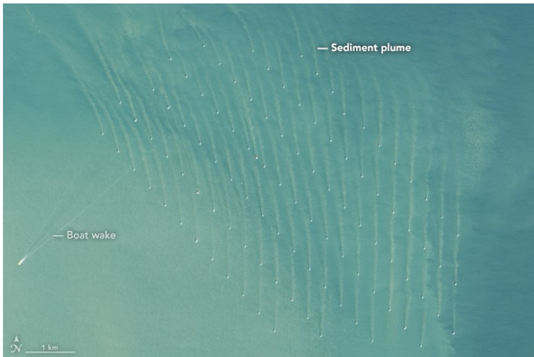
Figure 1.4. Sediment plumes at Thanet offshore wind farm viewed from space, white dots are wind turbines (photo credit: NASA Earth Observatory)
