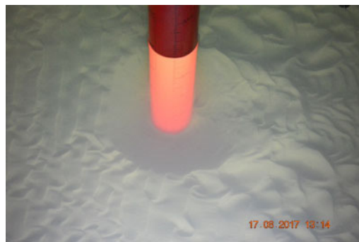
Figure 11. Local scour pit formed around the model monopile. From Test 6 in the Fast Flow Facility.
