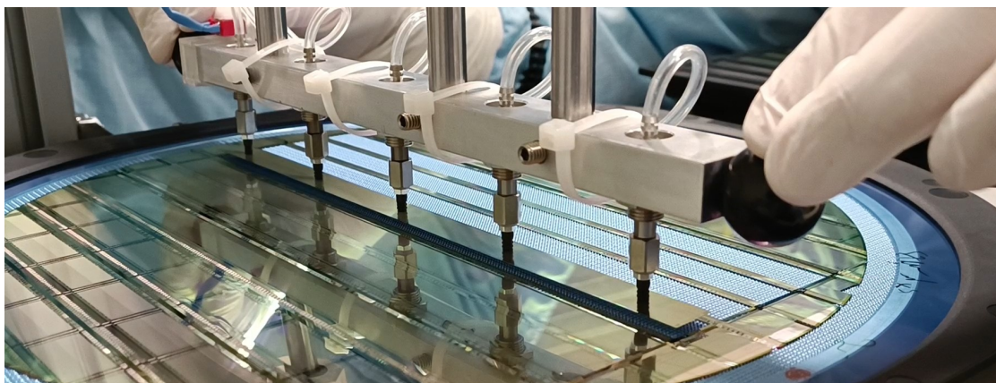
Figure 4.1: Picture of the pick-up system with annotated components (a), and in use (b). (c) Close-up view of the pick-up bar featuring five bellowed vacuum suction cups mounted on a spring-loaded and vertically travel-limited bar, used to safely pick up the chip.
