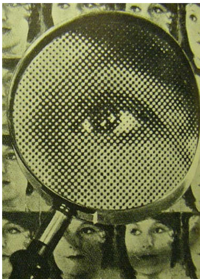
Fig. 2-17 'Dots' on a halftone screen. Illustration taken from Jan Poortenaar, The Technique of Prints (1933), Fig. 80
