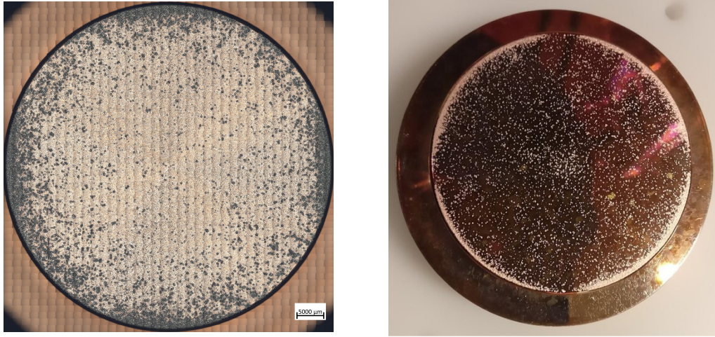
Figure 2.69: Images of 60 mm diameter DC electrodes after testing, both showing breakdown craters concentrated on the edges of the electrodes and grouped into four islands. Left: Tested at CERN, with breakdown craters appearing as dark points [87]. Right: Tested at the University of Helsinki, with breakdown craters appearing as white points [88].
