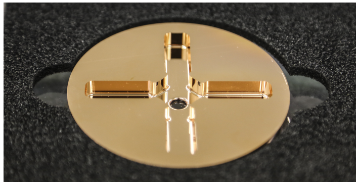
Figure 1.3: A copper disc containing a single cell with wakefield damping features.
