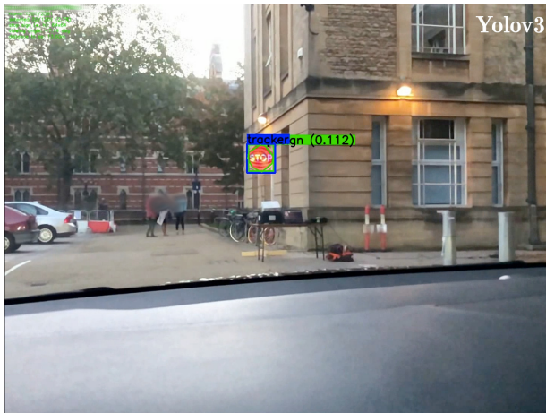
Figure 14: Sample video frame extracted from the outdoor experiment, for the 120 lux setting. The image shows the stop sign undetected under the threshold set in the experiments. The blue ‘tracker’ box is set manually and tracks the location of the sign.
