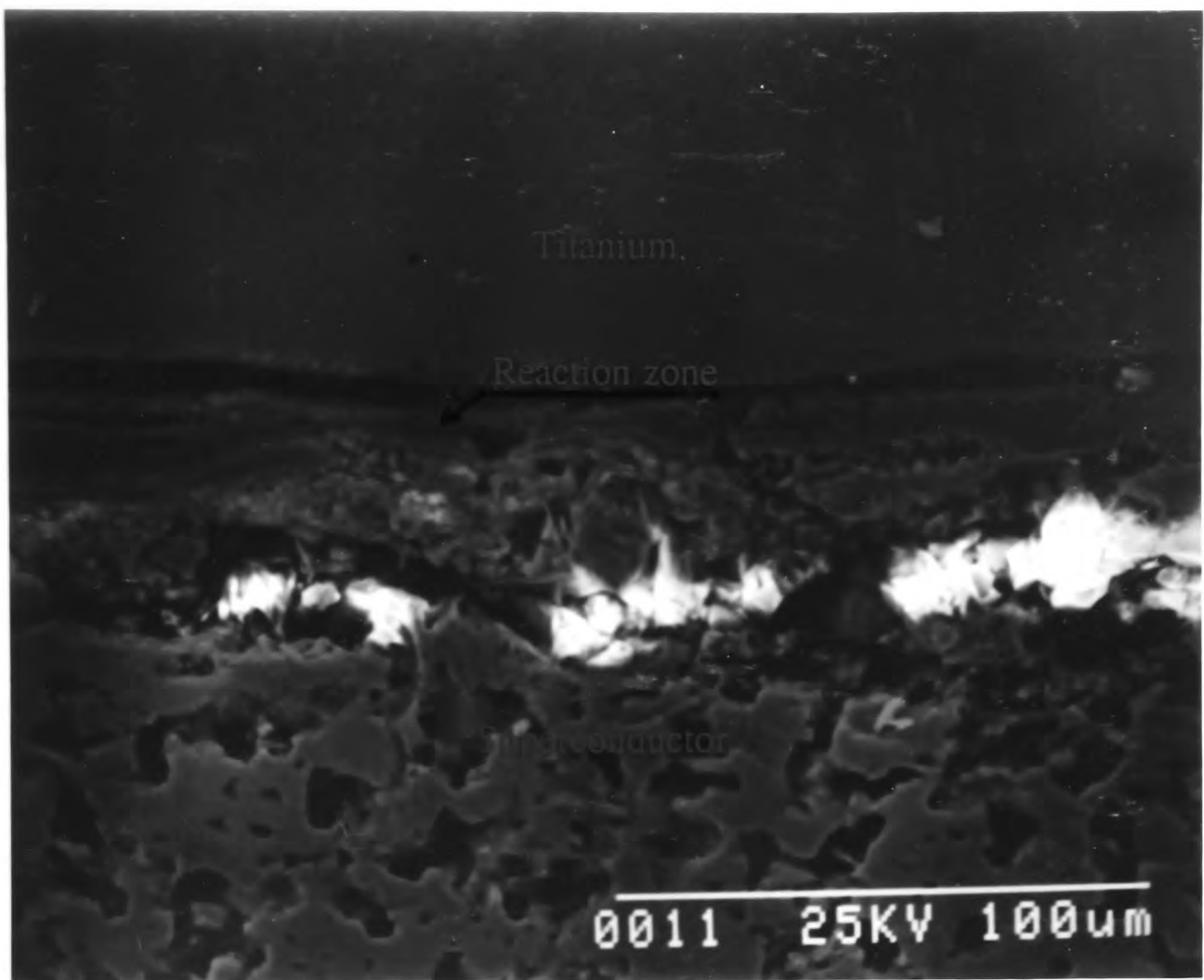
Figure 6.14: Interface of Ti/superconductor diffusion couple OS
