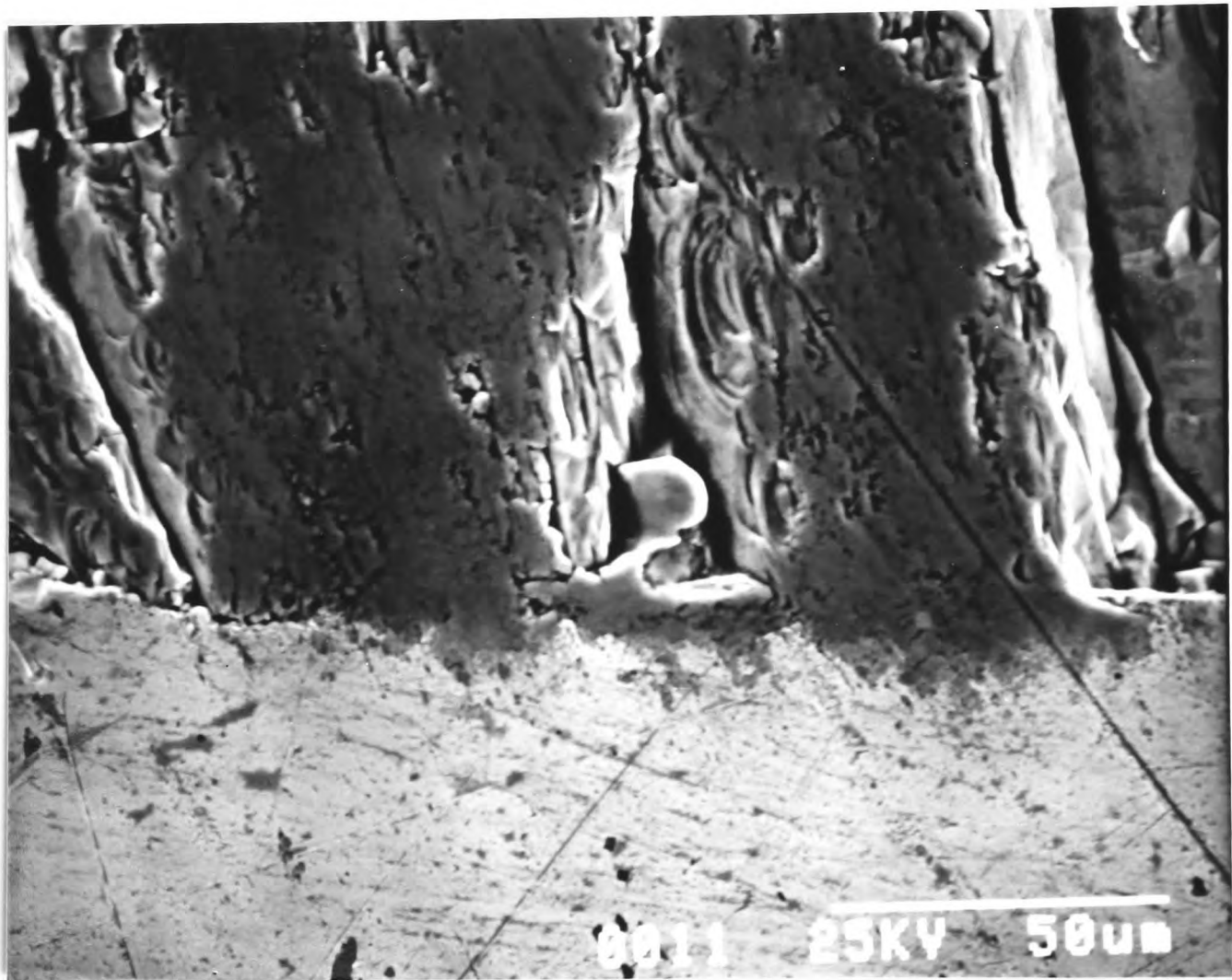
Figure 6.31: Interface of Au/superconductor MG
