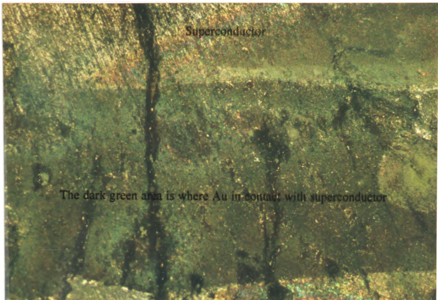
Figure 6.26a: Reaction products on superconductor surface MG
