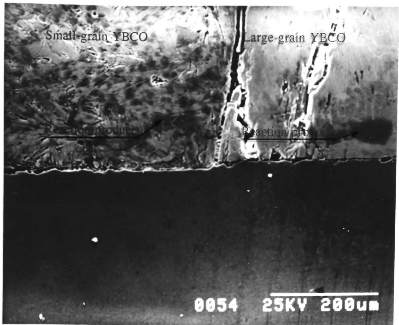
Figure 6.23: Interface of Pd/superconductor (annealed at 600°C for 1 hour) MG
