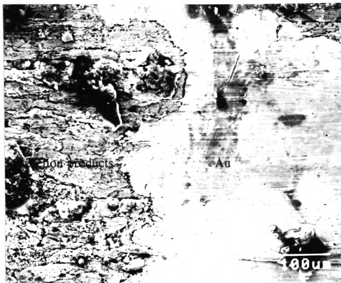
Figure 6.27: Reaction products on Au surface
