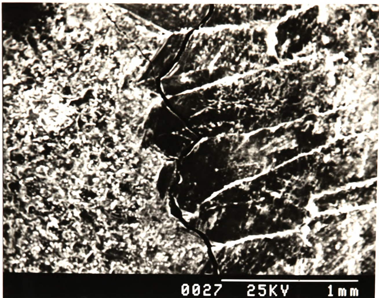
Figure 5.11: A crack source in a \text{YBa}_2\text{Cu}_3\text{O}_{7-x} crystal
