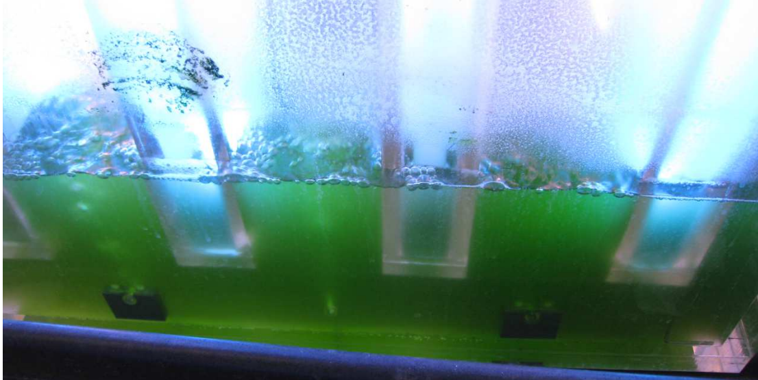
Figure 79. Bubbling differences in the photobioreactor on Day 60 of growth. The slightly higher gas flow rate in the left side of the tank may have caused a slight build-up of algae at the right end. However, the PBR was well mixed before sampling.
