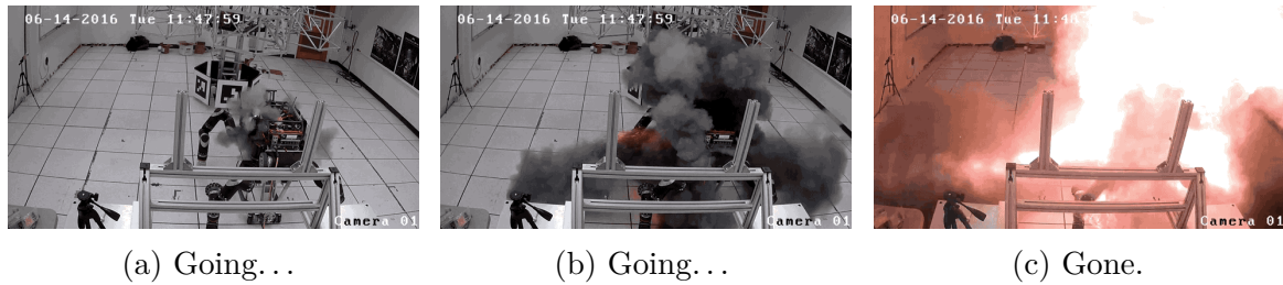
Fig. 1.1: Battery management failure of a RoboSimian droid at the Jet Propulsion Laboratory [21].
