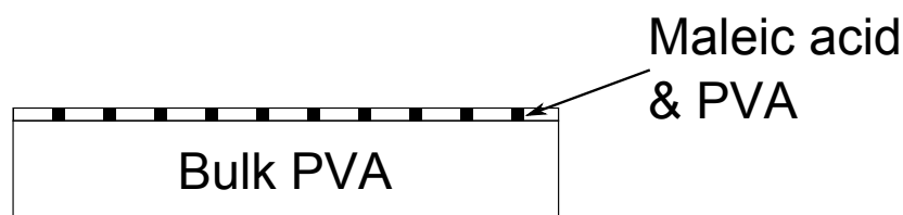
Figure 5.19: Idealised PVA and maleic acid film cross-section prior to annealing.
