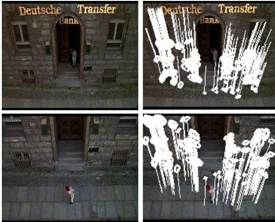
Fig. 10. Detail of matches for key frames 4 & 9. Note the large motion vectors resulting from the change in camera elevation between shots – only one half of each image overlaps with the other.
