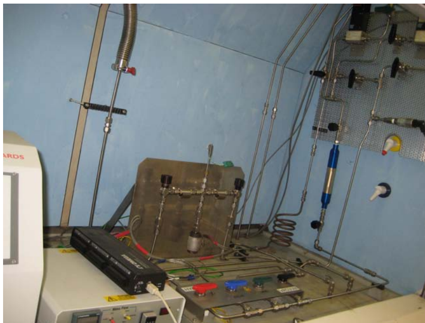
Figure 2.15: Photograph of the author's custom built hydriding apparatus. On the lower left of the photo, the electronic controls and data acquisition box can be seen.
