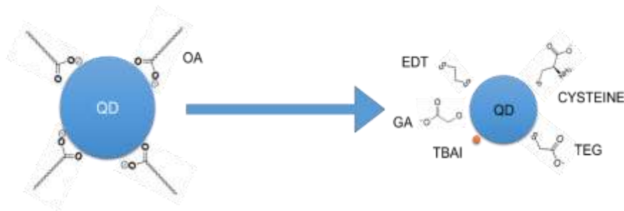
Figure 4.2: Schematic illustration of a ligand exchange process replacing the long-chain oleic acid (OA) with smaller molecules such as TBAI, EDT, GA, TEG, and Cysteine.
