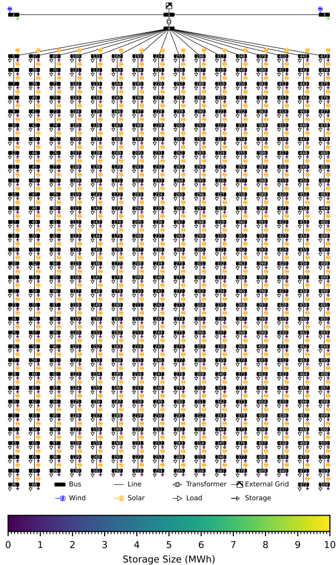
Figure 5.20: Storage size and placement determined using the proposed method with DC OPF in the carbon-neutral village. Larger storage units are placed on buses hosting wind turbines, while smaller storage units are placed on the 500 prosumer buildings with solar PVs.
