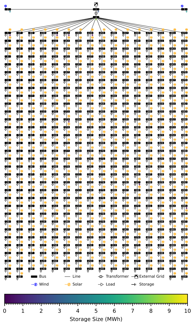
Figure 5.21: Storage size and placement determined using the proposed method with AC OPF in the carbon-neutral village. Larger storage units are placed on choke point buses before and after the transformer, as well as on buses hosting wind turbines. Smaller storage units are placed on prosumer buildings with a larger difference between generation and demand.
