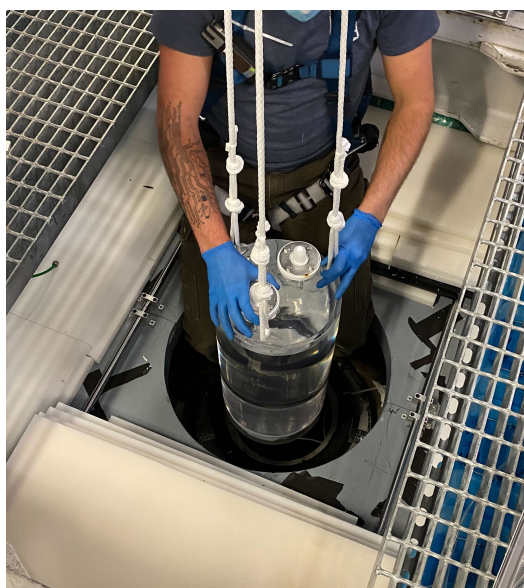
Figure 22. Deployment of the GdLS plug — a small cylindrical acrylic tank with neutral buoyancy. It is used to fill the cut-out during the science run and is only replaced with the YBe source during calibrations.
