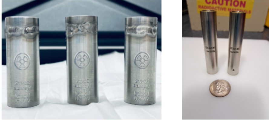
Figure 13. Left: three custom-made AmLi sources used in LZ. The gold-americiam-lithium matrix is encapsulated in nested tungsten and stainless steel capsules, which are designed to integrate with the CSD system and provide gamma-radiation suppression. The welds on the outer stainless-steel capsules are visible in the picture. Right: two customized AmBe sources from Eckert & Ziegler designed for LZ. The stainless steel threaded capsules were designed to integrate in the CSD system and shield against low energy gammas from ^{241}\text{Am} decay.
