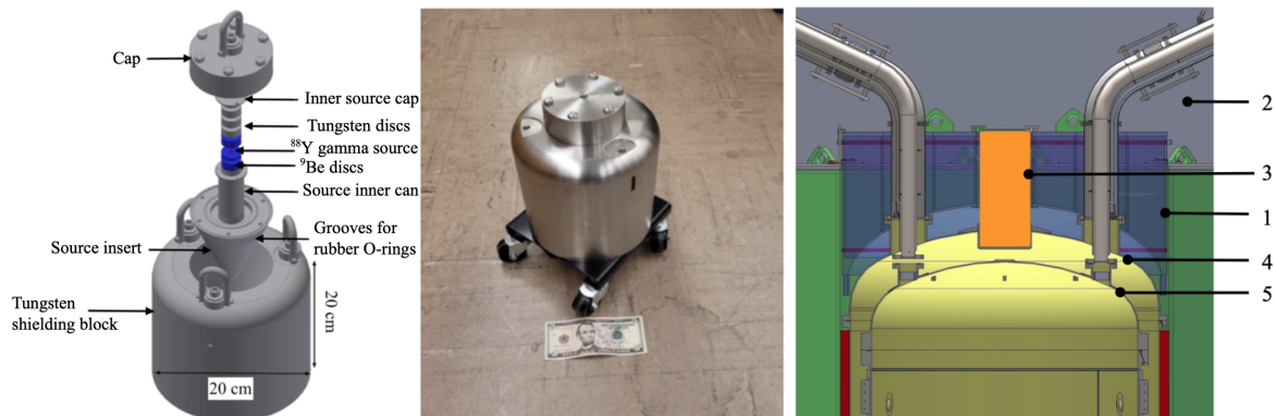
Figure 21. Left: CAD drawing for the YBe photo-neutron source assembly. The ^{88}\text{Y} sealed source is sandwiched between ^9\text{Be} disks to generate neutrons. The tungsten shielding reduces the number of ^{88}\text{Y} \gamma -rays that can enter the detector. Middle: YBe source inside the tungsten shielding placed next to a five-dollar bill for scale. Right: layout of the top part of the OD (1, including both the green and purple volumes) and water tank (2). The custom cut-out (3) in the OD acrylic vessels through which the YBe source is deployed is shown. The OCV (4) and ICV (5) are also indicated in the figure.
