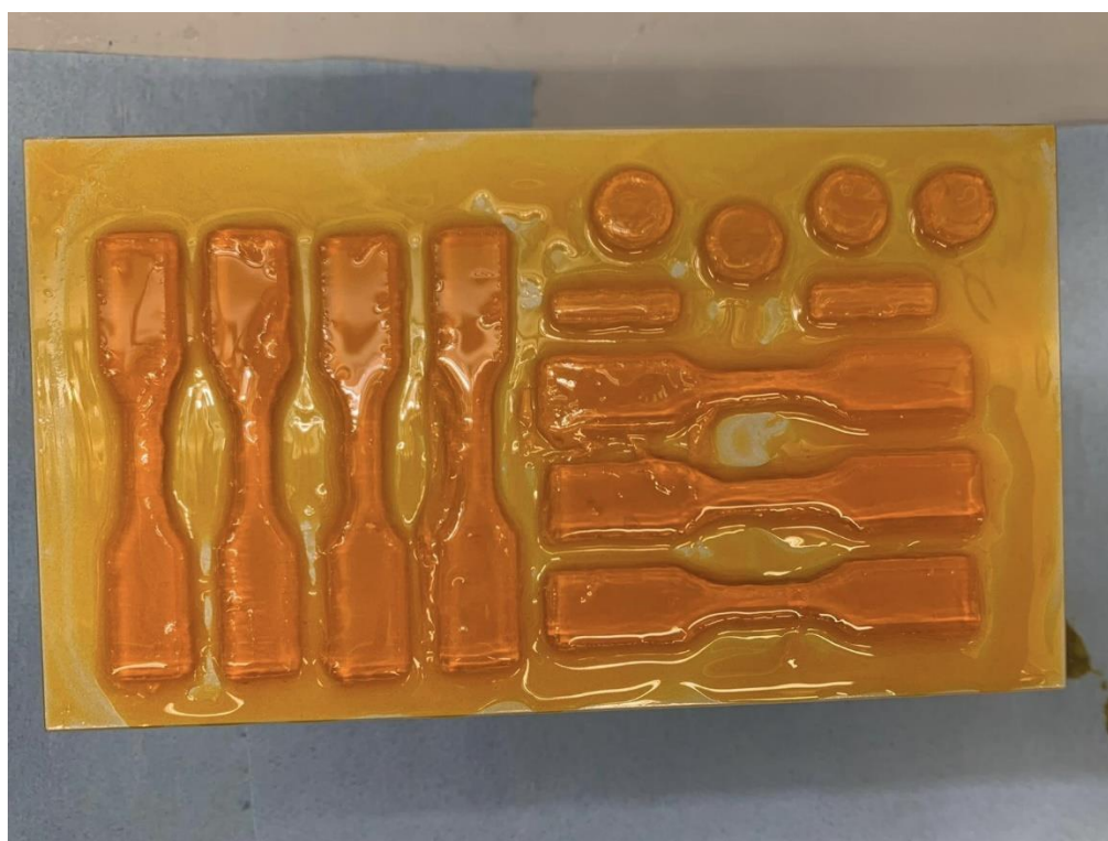
Figure 4.7: Digital photograph of P1X1 printed parts on built plate (before workup).
