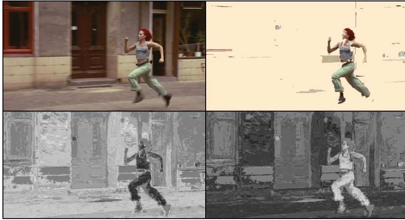
Fig. 4. Image segmentation with max-marginal probabilities. The first image is a frame of the movie Run Lola Run . The second shows the binary foreground-background segmentation where the aim was to segment out the human. The third and fourth images shows the confidence values obtained by our algorithm for assigning pixels to be foreground and background respectively. In the image, the max-marginal probability is represented in terms of decreasing intensity of the pixel. Our algorithm took 1.2 seconds for computing the max-marginal probabilities for each latent variable label assignment. The time taken to compute the MAP solution was 0.3 seconds.
