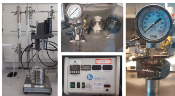
Figure 7.2. Pictures of the drying columns (L.H.S. picture), the high pressure reactor disassembled (upper middle picture), the high pressure reactor assembled (R.H.S picture) and the controller unit (lower middle picture) used for high CO 2 pressure polymerization.
