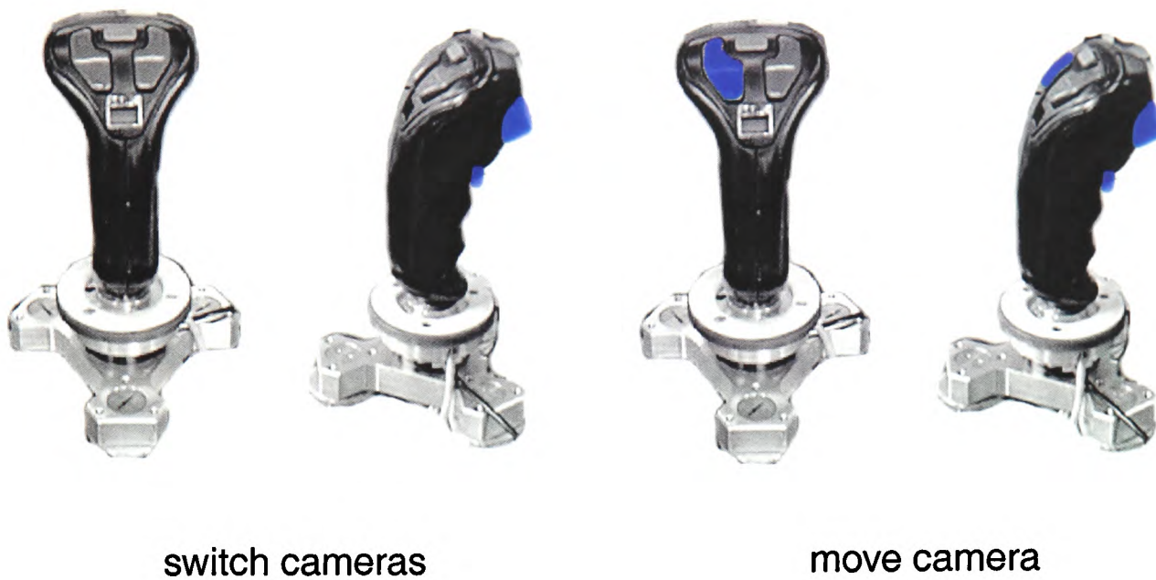
Figure 3.4: An example of the user interface : The operator can use the joysticks buttons to change teleoperation mode. When the trigger button is depressed a camera switch event is emitted. When both the re-index and trigger buttons are depressed a camera move event is emitted and the master input device can be used as a camera positioning tool.
