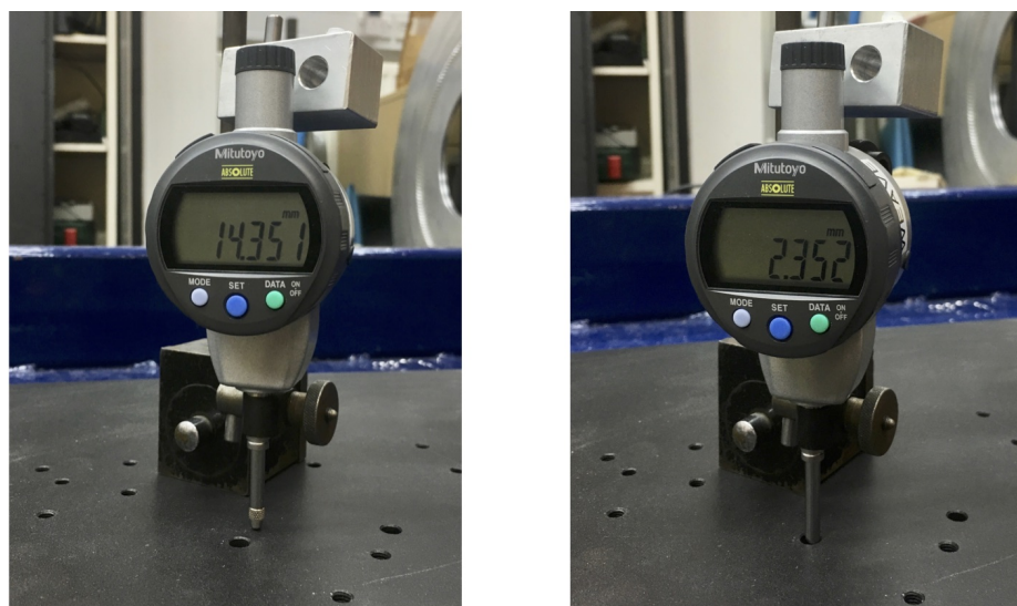
Figure 3.7: Two example readings of the interface plate. On the left a reading on top of the plate, on the right a reading through the hole, with the gauge touching the plate below. Not shown are the weights on either side of the measurement site.
