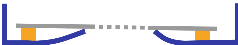
Figure 3.5: Side view of trolley in blue, old interface plate in grey, and shims in orange. Note that the plate is flat but not necessarily horizontal. This does not matter for the measurements as everything is measured with respect to the interface plate. This situation assumes that the interface plate bends back under the positioner's weight.
