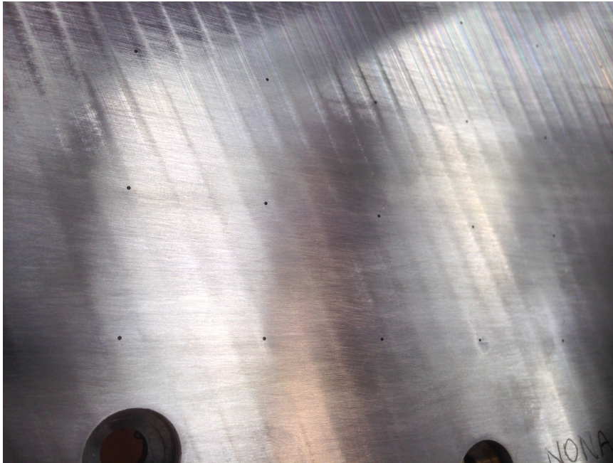
Figure 4.2: A close-up of the grid machined into the prototype field plate, in this case made of aluminium. Each point is 0.5 mm wide, and the ones visible here are filled with black paint and lightly sanded.
