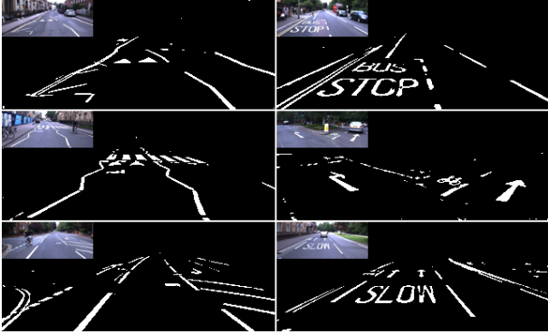
Fig. 3. Road marking detection performed by a deep semantic segmentation network in real-time. Before the detections are employed to generate the scene graph, they are mapped to top-down view.
