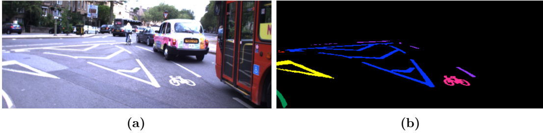
Figure 4.3: The road markings are classified semantically and displayed in different colours, (b), for a complex urban intersection, (a). We ideally retrieve this mapping directly from the image and include the result in the scene graph to guide planning and decision making.
