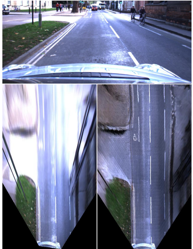
Fig. 1. Boosted Inverse Perspective Mapping (IPM) to improve the understanding of road scenes. Left : Top-down view created by applying a homography-based IPM to the front-facing image ( top ), leading to unnatural blurring and stretching of objects at further distance. Right : Improved top-down view generated by our Incremental Spatial Transformer GAN, containing sharper features and a homogeneous illumination, while dynamic objects (i.e. the two cyclists) are automatically removed from the scene.
