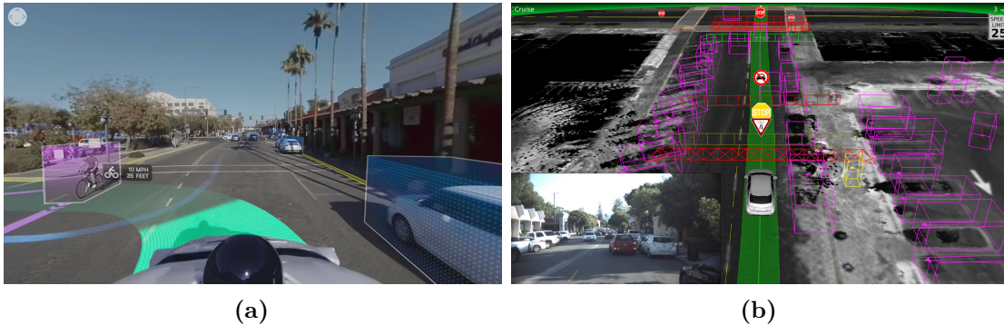
Figure 1.1: Autonomous vehicles have to manoeuvre through complex road layouts shared by different types of traffic participants in urban environments, (a). The mediated approach builds a representation which describes all relevant (road) objects in its environment and can be employed for decision making, (b). Photographs (a) and (b) courtesy of Waymo.
