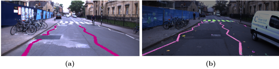
Figure 6.3: When the conditions are favourable (i.e. bright, newly-painted road markings on dark tarmac), the model-driven, (a), and the data-driven approach, (b), both accurately classify all the pixels belonging to the zig-zag road marking instance of interest.
