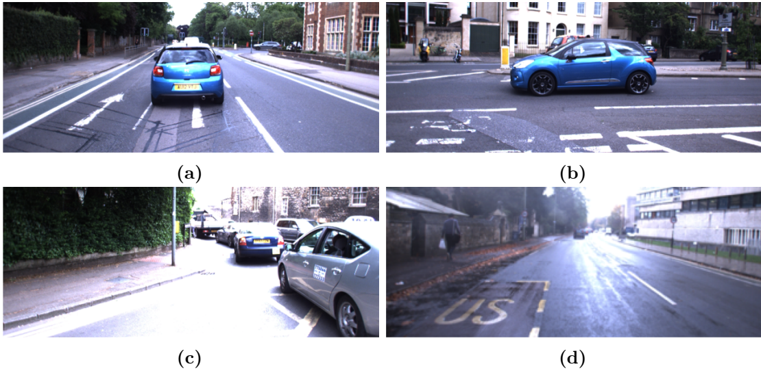
Figure 5.2: Road marking segmentation is challenging for several reasons such as occlusions, (a), degradation, (b), overexposure, (c), or combinations of these, (d). Heuristic methods most likely fail under these circumstances. DNNs might resolve these limitations when adequate training data is available and by using the global scene context.
