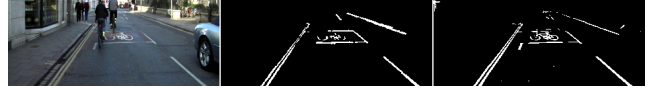
Fig. 7. The CamVid label ( middle ) and the predicted output ( right ) for a test image. The predicted output reflects the ground truth better at several places in the images such as the lower part of the bounding box around the bicycle and the bicycle itself.
