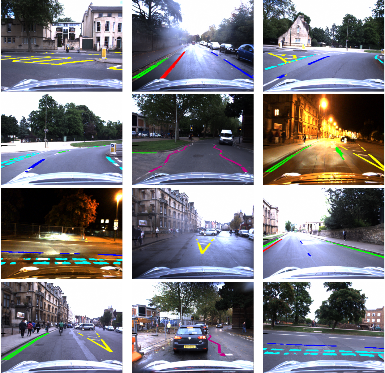
Fig. 5. Sample of results from the semantic classification of road marking pixels under different weather and lighting conditions (overcast/rain/night). By using a global energy approach, our proposed approach is able to detect multiple road marking segments in images from detected road marking pixels. These segments are aggregated through another energy minimisation into their semantic classes. Thereby, we reveal the underlying meaning of the road markings in complex urban environments, providing important cues for autonomous vehicles. These include indication for upcoming road situation, which could require specific behaviour. For instance, the zig-zag markers ( purple ) indicate an upcoming pedestrian crossing and the give-way dashes ( cyan ) indicate a junction.
