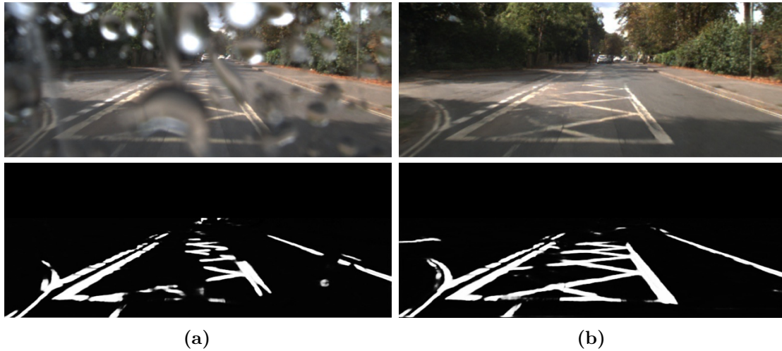
Figure 5.7: Raindrops and water streaks adherent to the lens significantly distort the view and consequently the segmentation performance, (a). The image is de-rained by an image-to-image translation network and the road marking segmentation is thereby restored, (b).
