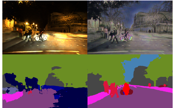
Fig. 1. Our method allows off-the-shelf models to work with new, unseen domains, without any specific fine-tuning. In this example, we use our input adapter to allow a segmentation model trained using only daytime examples to work under night-time conditions. Top-left quadrant is the input night-time image, top-right quadrant is the output of our input adapter. The bottom-left quadrant is the output of the segmentation model applied on the original night-time input image. The bottom-right quadrant is the output of the segmentation model applied on the output of our adapter. The initial segmentation result is unusable, while the result obtained by running the model on the output of our domain adaptation pipeline accurately classifies roads, pavement, pedestrians, bicycles, vegetation and buildings.
