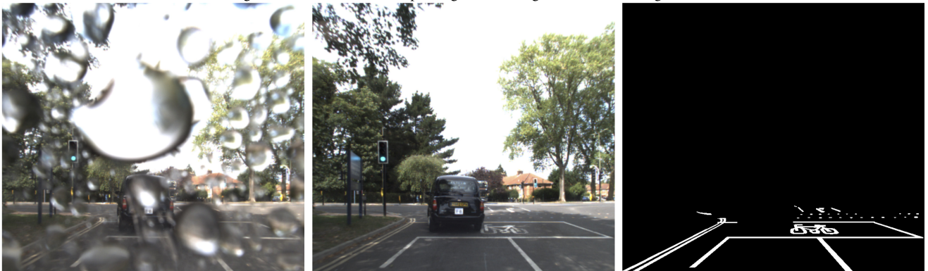
Fig. 7. An example from our stereo dataset. The image on the left is produced by the left lens, which is affected by water drops. The image in the middle is produced by the dry right hand lens. The image on the right is the road marking segmentation ground truth.
