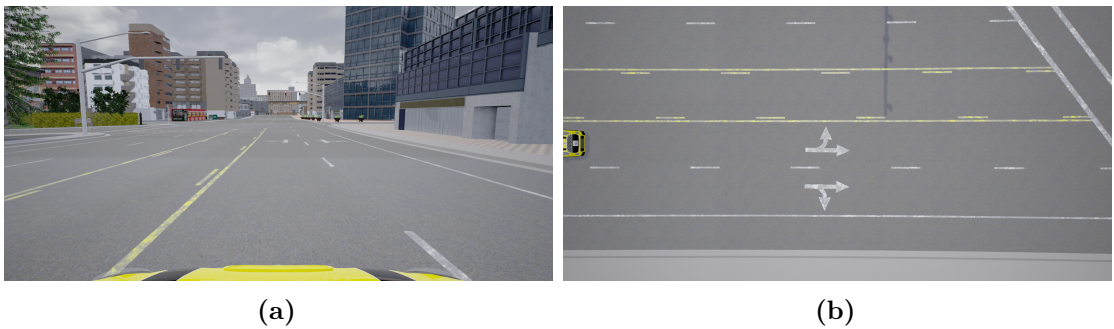
Figure 2.5: An example of a bird’s-eye-view training pair in the CARLA simulator. The camera position is adjusted to retrieve a ground-truth bird’s-eye view (displayed at a 90° rotation), (b) , aligned with the front-facing camera image, (a) .
