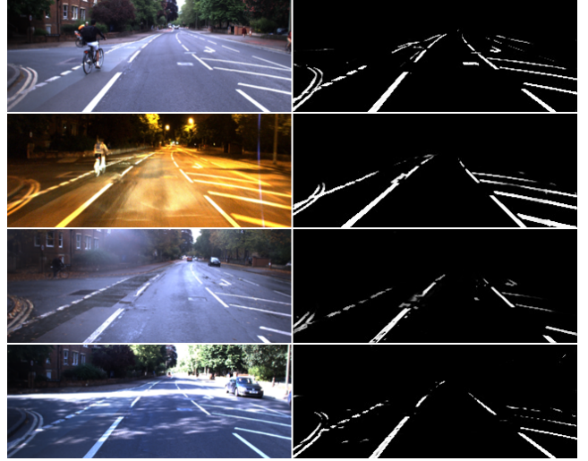
Fig. 2. Road marking detection under different lighting conditions (overcast, night, rainy, and sunny). Despite the large changes in the prevailing conditions the trained deep segmentation network [4] is able to accurately identify the pixels belonging to the road markings from the monocular image.
