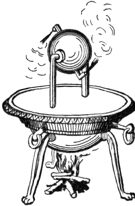
Figure 1.1: Hero's Steam-Engine or aeolipile as drawn in Knight's American Mechanical Dictionary [69].
