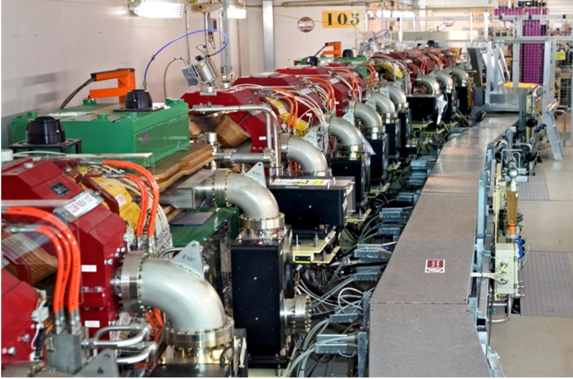
Fig. 2.3: Diamond Light Source cell showing magnets that make up magnetic lattice mounted on a support girder.
