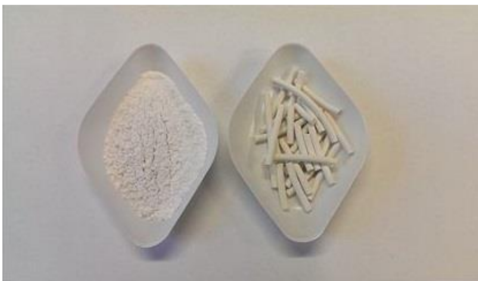
Fig. 4.1b 1g nano \text{H-ZSM-5} ( \text{Si/Al}=60 ) powders (left) and 5g extrudates (right)
