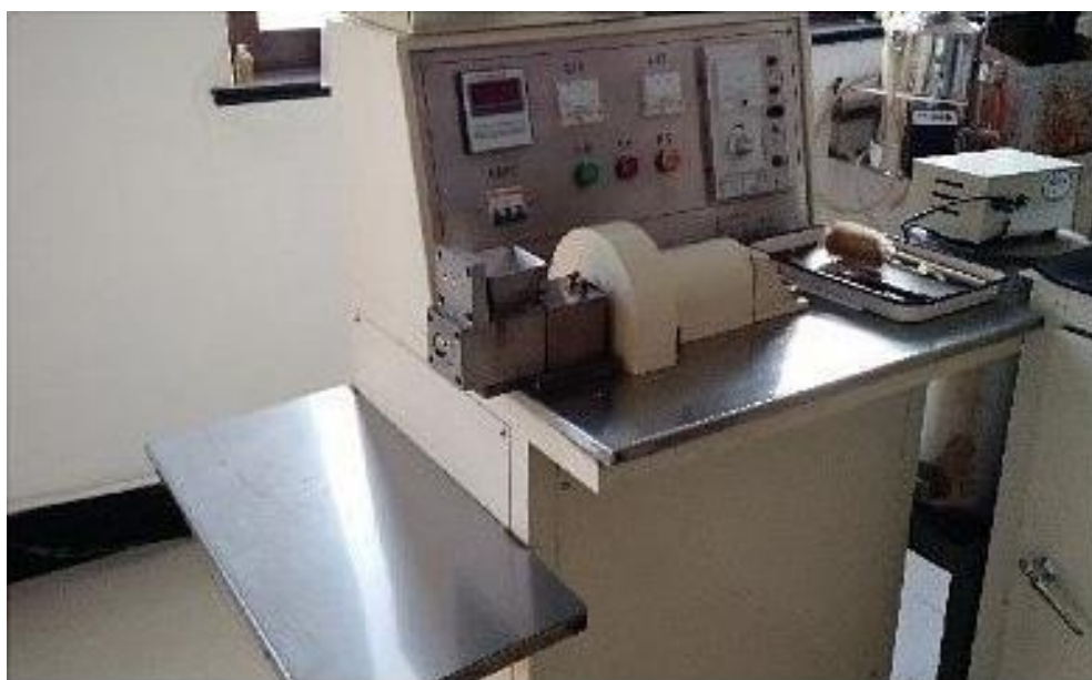
Fig. 4.1a mini screw extruder employed for catalyst shaping
