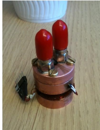
(b) Bobbin 2- Commercial 50 ohm load soldered into bobbin.
