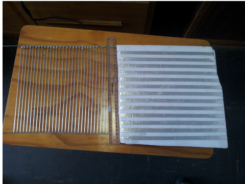
(a) Two polarizing grids made out of welding rods (Left) and aluminium tape (Right).
