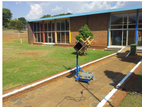
(b) The transmit horn was rotated to change the polarization of the test signal
