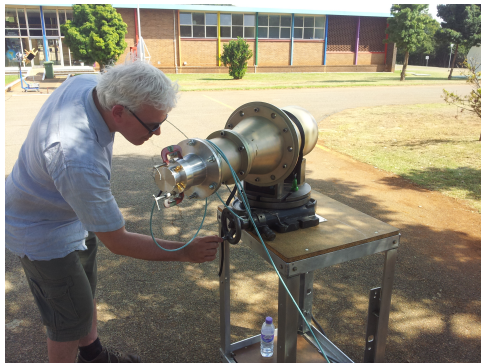
(a) The OMT was clamped onto the horn transition section and rotated to align it with the transmit horn polarization
