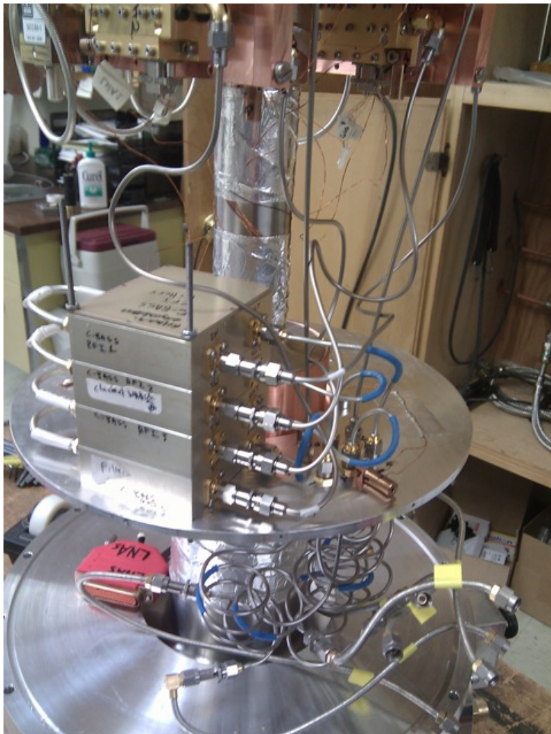
Figure 2.6: The notch filters installed in the cryostat at Owens Valley.
