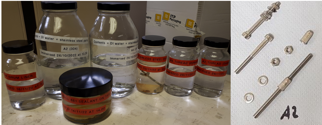
Figure 12.5: Photographs of the soak testing procedure. Left: stainless steel, tank and drum liner materials are immersed in DI water, held within separate jars at room temperature. Right: A2 grade steel components are shown upon completion of the testing process.
