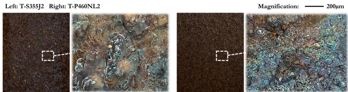
Fig. 4. Morphology of rust layers on carbon steel in Knokke-Heist after year-long exposure.
