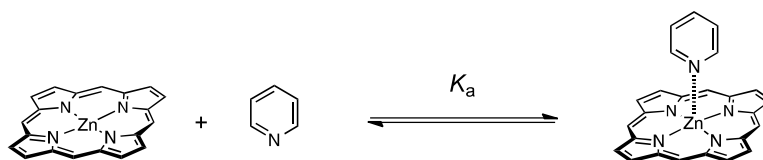
Figure 1.11 Binding of Zn porphyrin monomer with axial pyridine.
