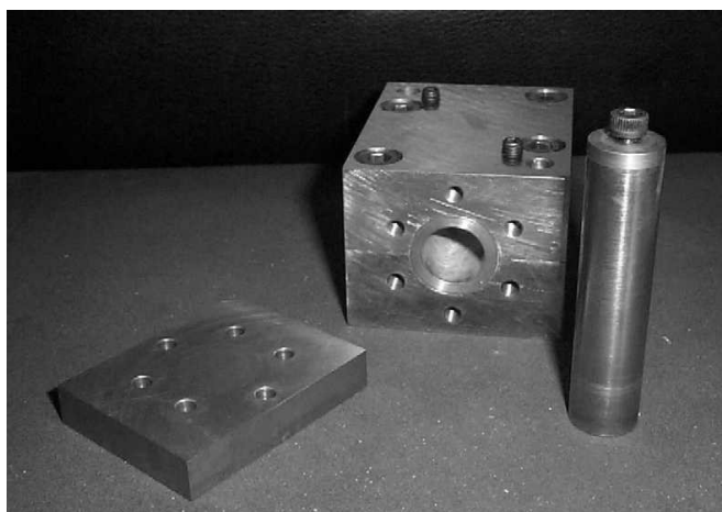
Figure A3:- Diepress for Uniaxial pressing of TE 01n Garnet Resonators
