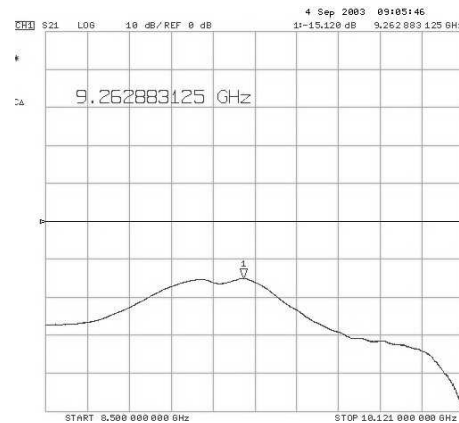
Figure 123:- Response of Unmagnetised 7.0738mm Long Microstrip Resonator on 0.4 Volume Fraction C4A Composite Substrate Designed Using Forward Measured T / R Properties
