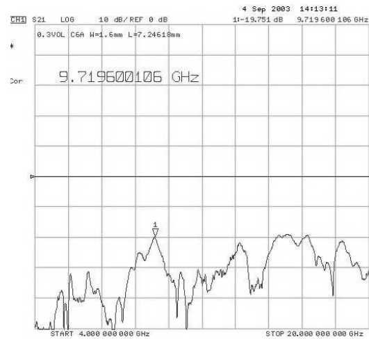
Figure 130:- Response of Unmagnetised 7.24618mm Long Microstrip Resonator on a 0.3 Volume Fraction C6A Composite Substrate
