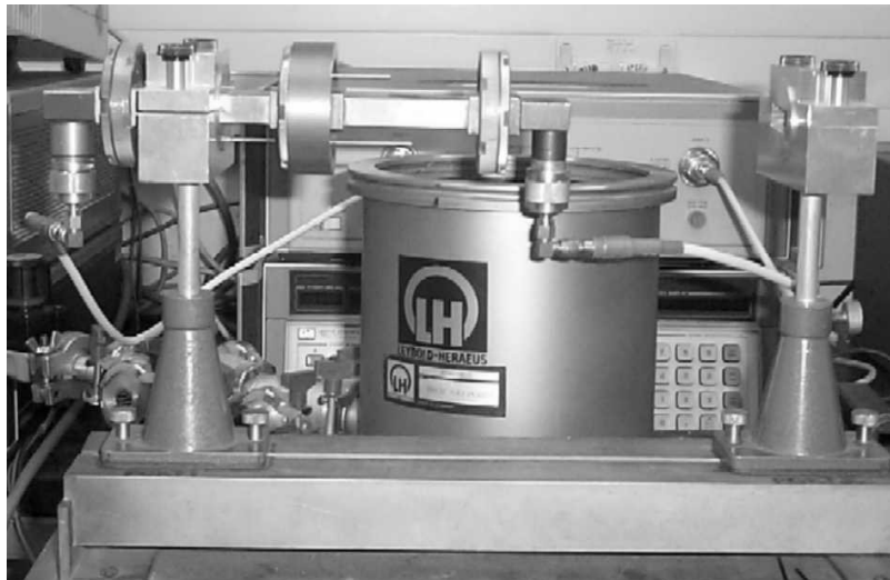
Figure 8:- WR90 Transmission / Reflection test setup
