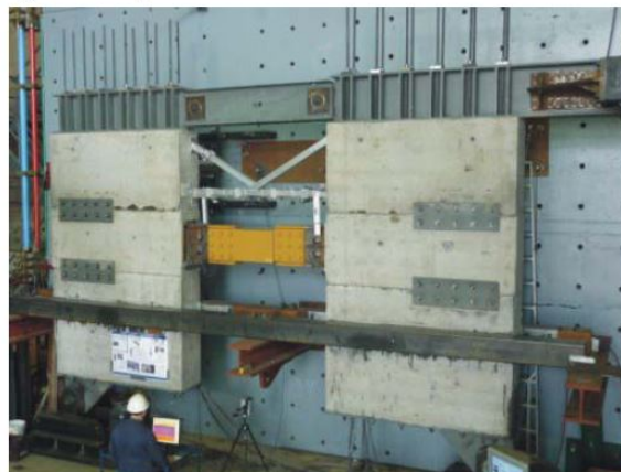
Figure 2.32: Experimental rig for VE dampers replacing coupling beams [38]
