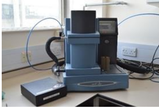
Figure 3.9: TA instrument DMA Q800 (university of Oxford, Engineering department)
