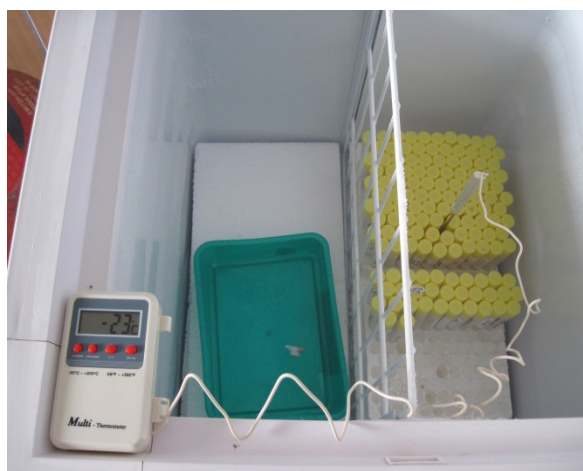
Fig. 20 Storage of saliva samples in a freezer (open view) below -20^{\circ}\text{C} .
