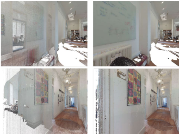
Fig. 4 Images from the left and right sides illustrate the before and after of rendered images from the point cloud when utilizing an adjustable point size based on the distance to the virtual camera
