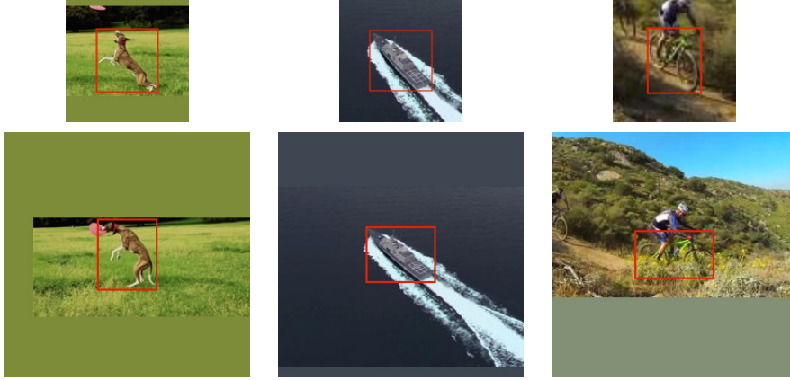
Figure 5.2: Pairs of training samples (exemplars z and corresponding search areas x ) extracted from the same video. When a sub-window extends beyond the extent of the image, the missing portions are filled with the frame’s mean RGB value.
