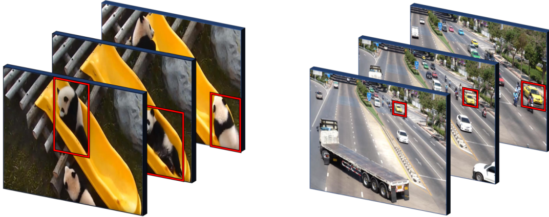
Figure 1.3: Arbitrary object tracking. Given the supervision of a rectangular bounding box identifying an arbitrary object in the first frame of a video, the problem is to estimate the object’s position in all subsequent frames. In many applications of video understanding, tracking is a fundamental component as it allows one to obtain semantic coherence between frames.
