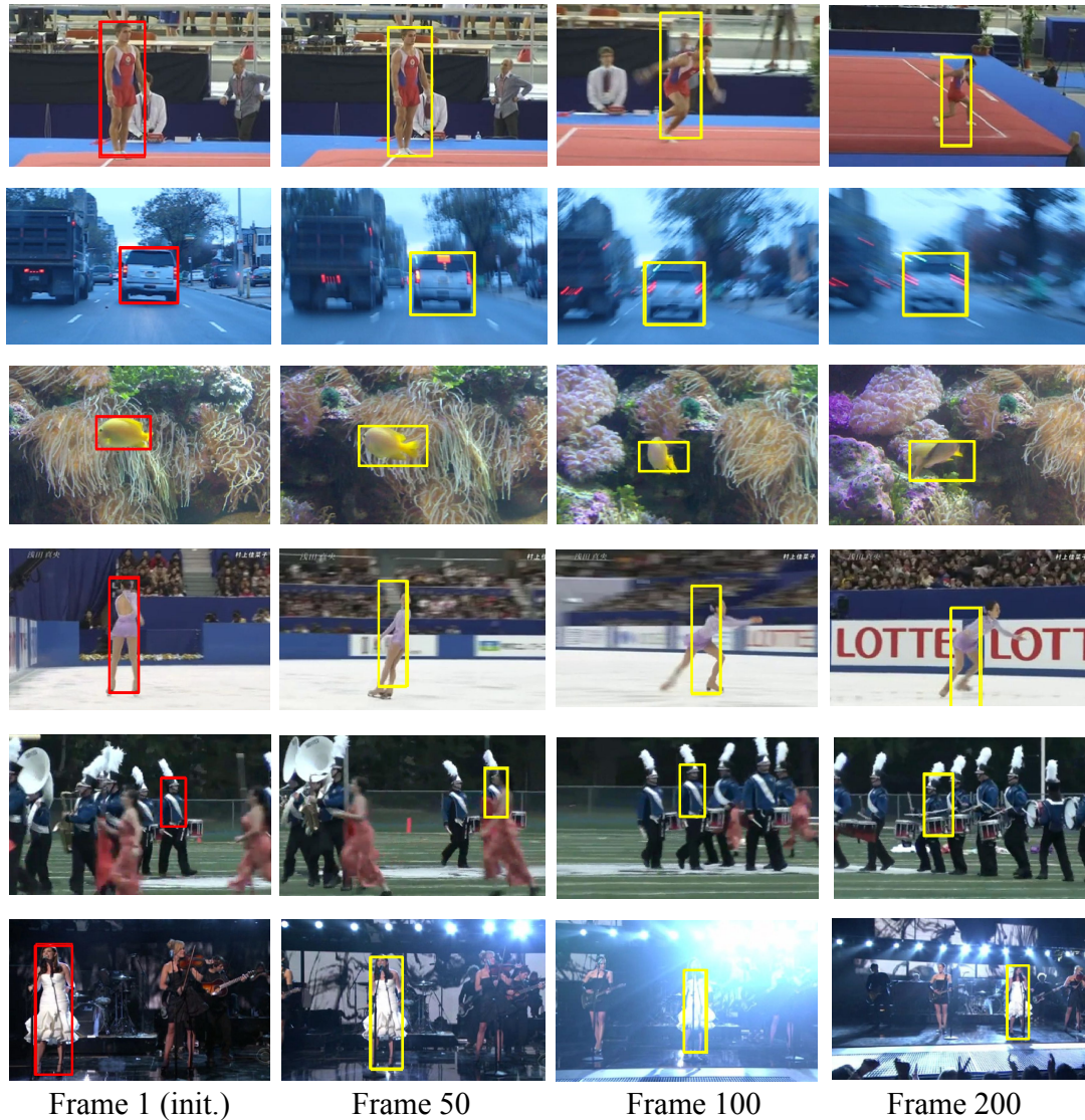
Figure 5.6: Snapshots of the simple SiamFC tracker described in Section 5.4 equipped with our proposed fully-convolutional Siamese network trained from scratch on ImageNet Video [184]. Our method does not perform any model update, so it uses only the first frame to compute \varphi(z) . Nonetheless, it is surprisingly robust to a number of challenging situations like motion blur (row 2), drastic change of appearance (rows 1, 3 and 4), poor illumination (row 6) and scale change (row 6). On the other hand, our method is sensitive to scenes with confusion (row 5). All sequences come from the VOT-2015 benchmark: gymnastics1 , car1 , fish3 , iceskater1 , marching , singer1 . The snapshots have been taken at fixed frames (1, 50, 100 and 200) and the tracker is never re-initialised.
