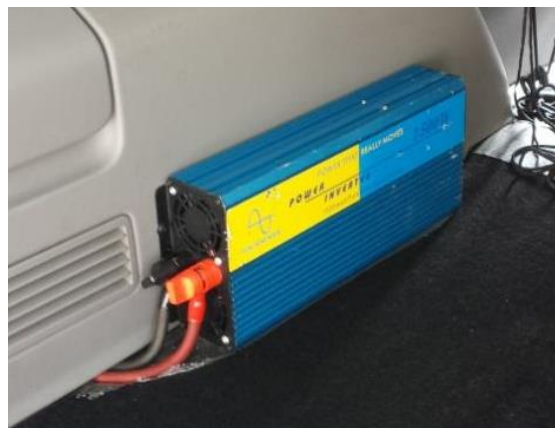
Image 12: DC to AC power inverter fitted in Amvale ambulance
