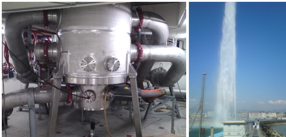
Figure 2.7: The resistive magnet (M10) at the LNCMI-Grenoble (left). At full field of 30 T the 20 MW magnet requires 300 litres of water per second for cooling the copper, comparable to the output of the 140 m high Jet d'Eau fountain in Geneva.
