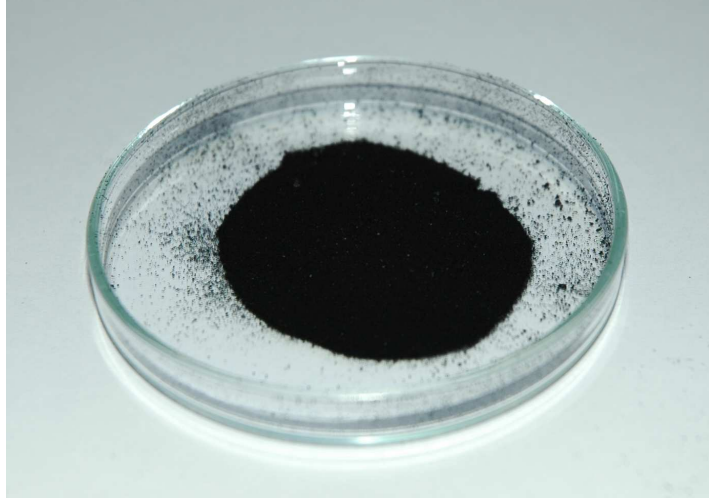
Figure 1.4: Macroscopic amounts of pure carbon nanotubes have the appearance of a fine black soot.
