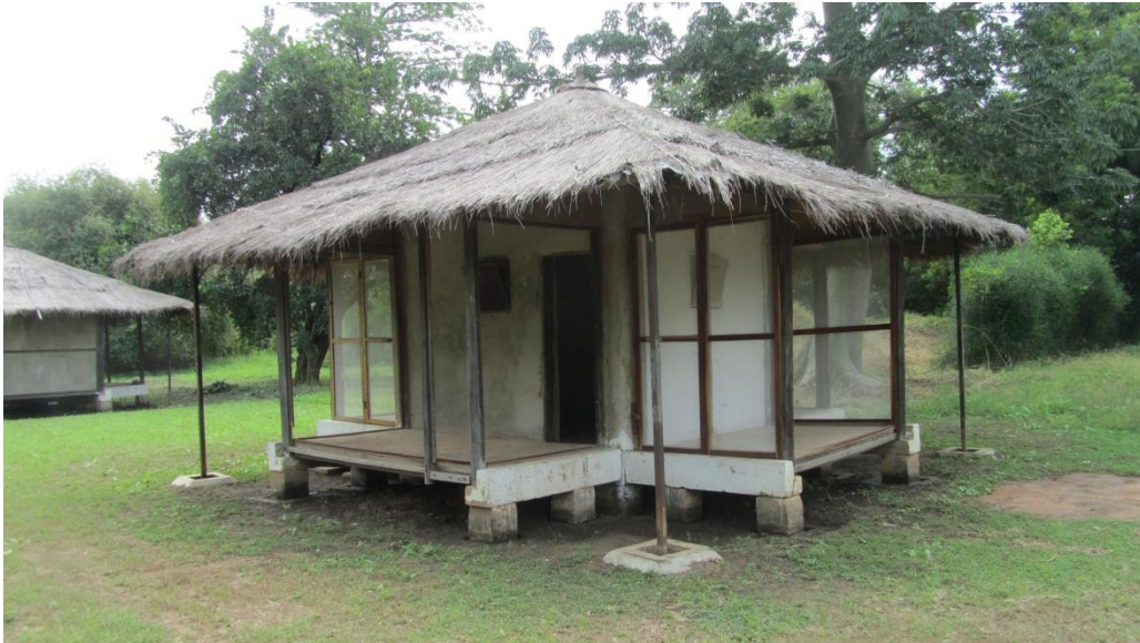
Figure 3.2. Experimental hut in Wali Kunda. The verandas were left open in order to allow mosquitoes to enter through the eaves and windows.
