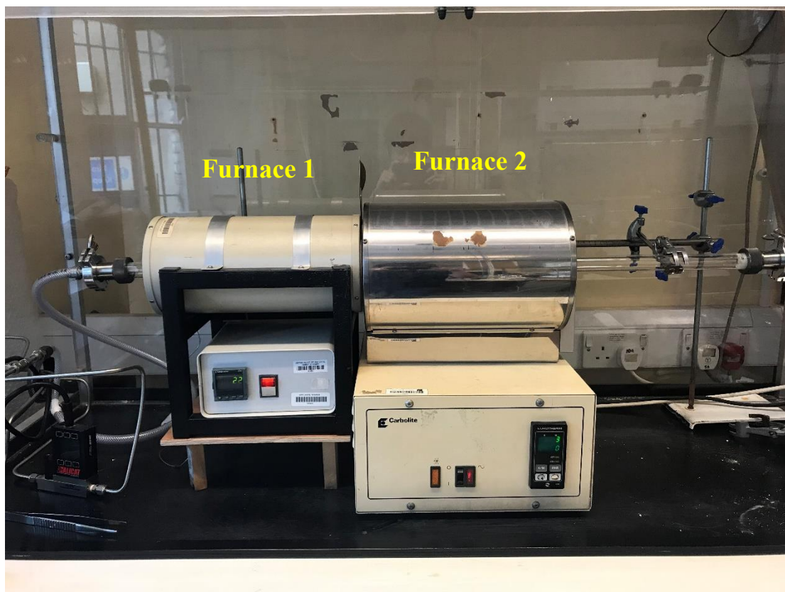
Figure 3.2. The CVD setup used for synthesis of MoS 2 , WS 2 and GaS in this thesis.
