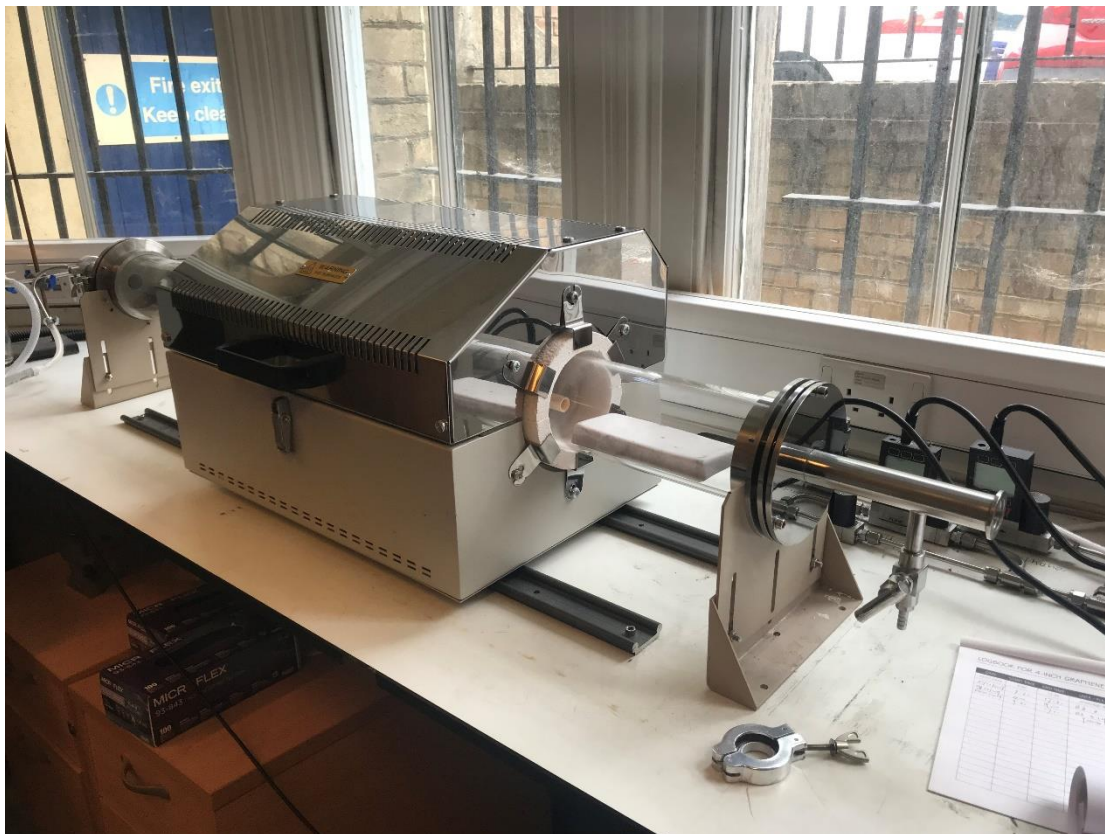
Figure 3.1. The CVD setup used for graphene synthesis in this thesis.
