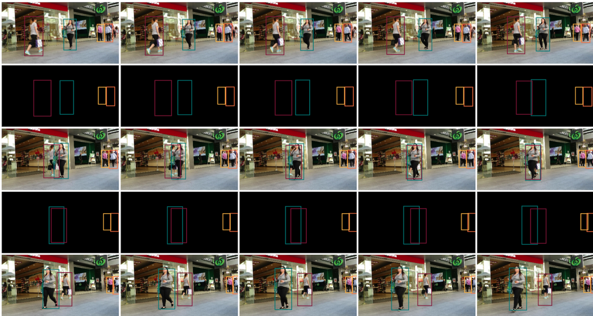
Figure 4.E.2: Camera blackout experiment on a pedestrian street scene from the MOTChallenge dataset without ego-motion. Subsequent frames are displayed going from top left to bottom right. Shown are the inputs to the model (some of them being black frames, i.e. arrays of zeroes) and bounding boxes predicted by MOHART (coloured boxes). This scene is particularly challenging as occlusion and missing sensor input coincide (fourth row).
