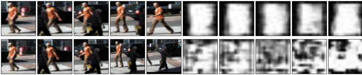
(a) The model with appearance attention loss (top) learns to focus on the tracked object, which prevents an ID swap when a pedestrian is occluded by another one (bottom).
