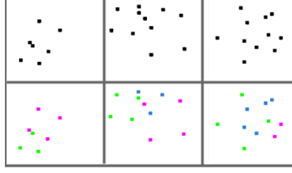
Figure 6.2.1: Unsupervised segmentation of points belonging to up to three constellations of squares and triangles at different positions, scales and orientations. The model is trained to reconstruct the points (top row) under the CCAE mixture model. The bottom row colours the points based on the parent with the highest posterior probability in the mixture model. The right-most column shows a failure case. Note that the model uses sets of points, not pixels, as its input; we use images only to visualize the constellation arrangements.
