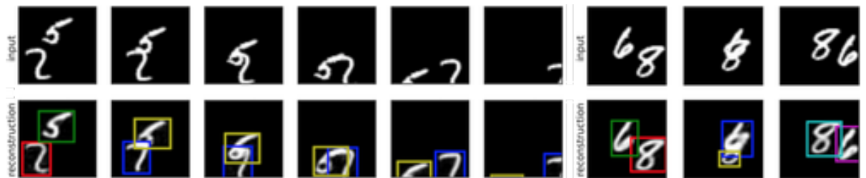
Figure 5.G.2: Examples of re-detections in MLP-SQAIR. Bounding box colours correspond to object identity, assigned to it upon discovery. In some training runs, SQAIR converges to a solution, where objects are re-detected in the second frame, and PROP starts tracking only in the third frame (left). Occasionally, an object can be re-detected after it has severely overlapped with another one (top right). Sometimes the model decides to use only DISC and repeatedly discovers all objects (bottom right). These failure mode seem to be mutually exclusive – they come from different training runs.
