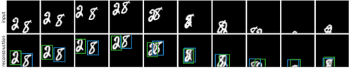
Figure 5.4.1: Input images (top) and sQAIR reconstructions with marked glimpse locations (bottom). For more examples, see Figure 5.H.1 in Section 5.H.
