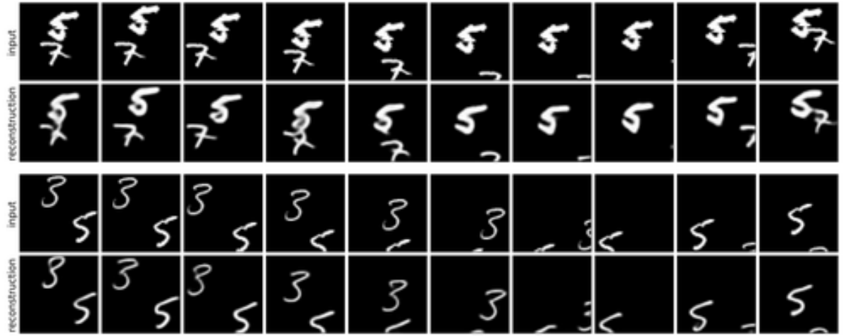
Figure 5.H.2: Sequences of input (first row) and CONV-VRNN reconstructions. They are not temporally consistent. The reconstruction at time t = 1 is typically of lower quality and often different than the rest of the sequence.
