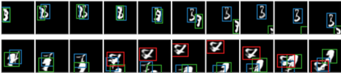
Figure 5.H.3: Samples from sQAIR. Both motion and appearance are temporally consistent. In the last sample, the model introduces the third object despite the fact that it has seen only up to two objects in training.
