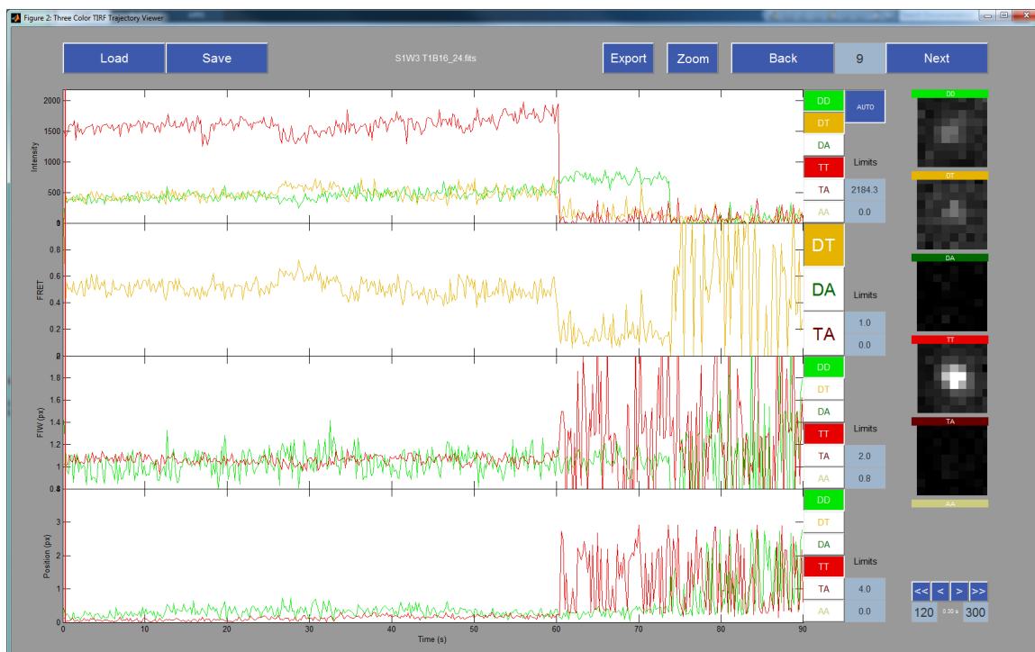
Figure 5.9: Timetrace viewer GUI. Once analysed, three-colour single-molecule timetraces can be displayed. The user can select which channels to display and can view the region of the movie corresponding to each frame in each channel.
