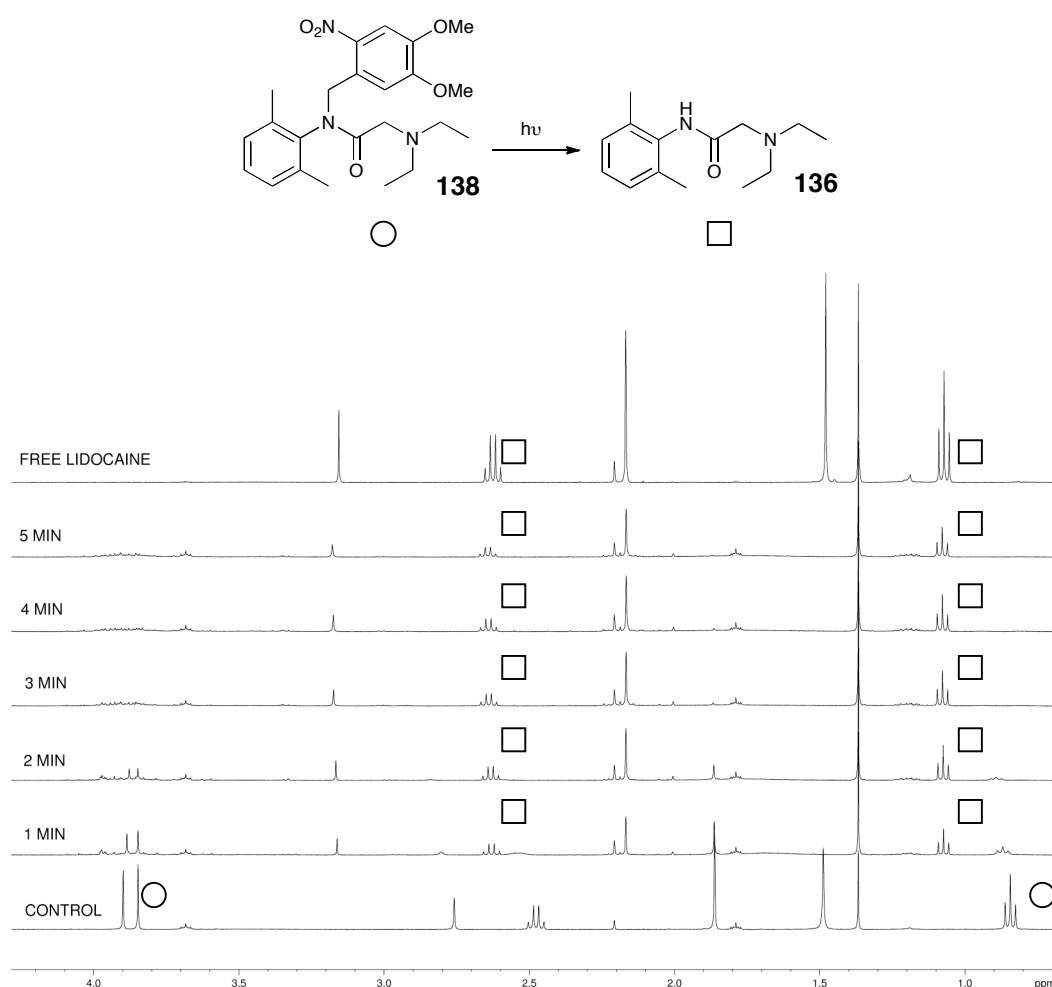
Figure 5.9. Partial 300 MHz ^1\text{H} NMR spectra in \text{CDCl}_3 of DMNB-caged lidocaine 138 photolysed at 25 mJ, 355 nm in THF for zero, 1, 2, 3, 4 and 5 minutes. Hexamethyldisiloxane standard in \text{CDCl}_3 was added to each sample after irradiation. The disappearance of peaks from the caged compound 138 ( \bigcirc ), including those at 0.85, 1.85, 2.50 and 3.85 ppm, and the appearance of peaks from what appears to be free lidocaine 136 ( \square ), at 1.10, 2.15, 2.65 and 3.15 ppm, were observed. The top spectrum is that of commercially available free lidocaine in the same NMR solvent. The peaks from this spectrum correspond to those which appear due to photolysis.
