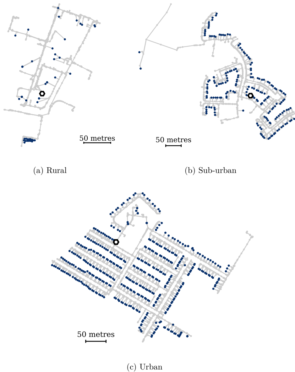
Figure B.1: The test networks used. Blue markers show the household locations and the black marker shows the substation position.
