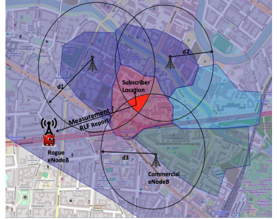
Fig. 7. Determining subscriber's precise location using trilateration (L3)
